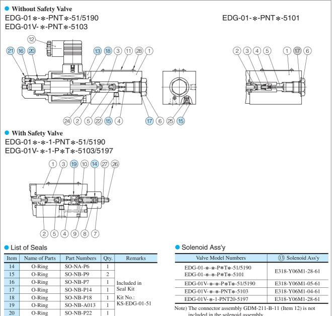
Note) O-ring (Item 16, 18, 20) and the fastener seal (Item 21) are included in the solenoid assembly.
