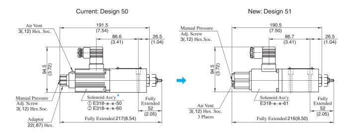
★ The solenoid assembly current design comes in two types: ① E318-50 design and ② 60 design. See the figure on the left for an external view of type ①. See the figure on the right for type ②.
